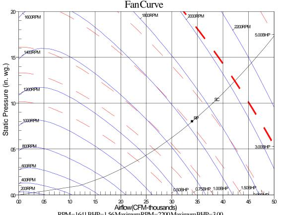
RPM=1641BHP=1.56MaximumRPM=2200MaximumBHP=3.00 SC-SystemCurve RP-RatedPoint
